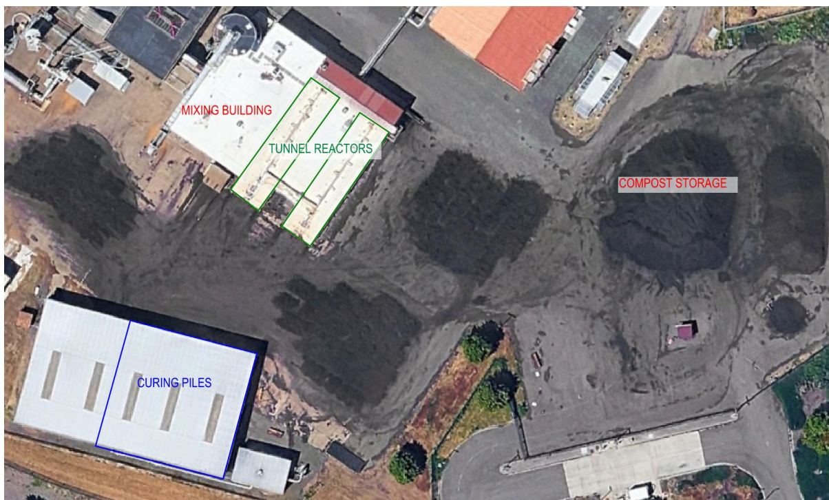
FIGURE 2-2: EXISTING COMPOSTING SITE LAYOUT
