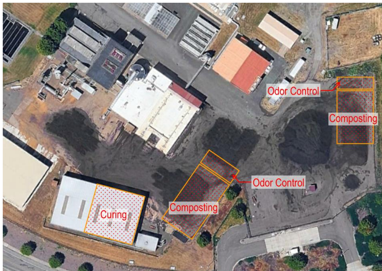
FIGURE 5-2: IN-VESSEL COMPOSTING SITE LAYOUT
