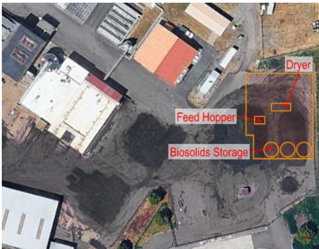
FIGURE 6-3: DRUM DRYER SITE LAYOUT
